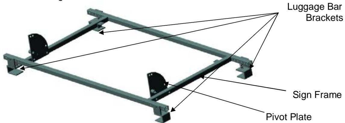
4. Mount the other side brackets using 3/8-16 x 2.0 inch bolts and 3/8-16 nuts.
